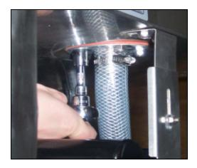
Removing the rinse drain weldment
